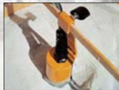
Dry probe: measures the level in the material hopper
