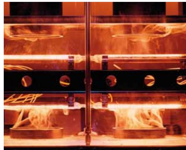
Plastic parts are simultaneously heated in two-sided modules and then welded together.
